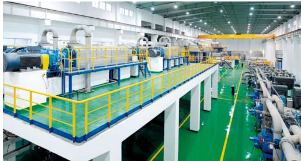
▲ The majority of the furnish is recycled fiber. Hebei has established wastepaper collection companies in Beijing, Tianjin, Harbin, and Shenyang. ANDRITZ delivered three stock preparation lines with a production capacity of 1,570 t/d and the approach system. ▶
