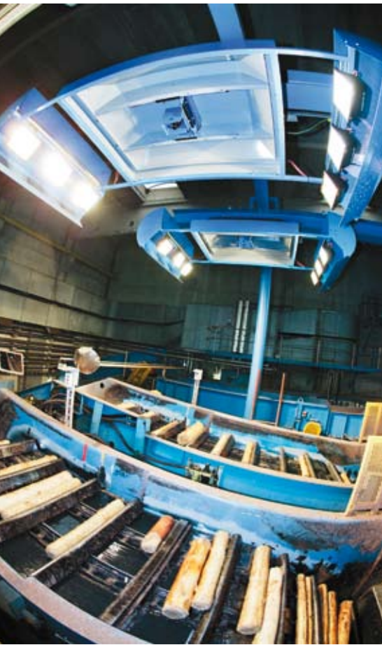
▲ LogScan™ uses a special video camera and light source mounted above the log conveyor.
