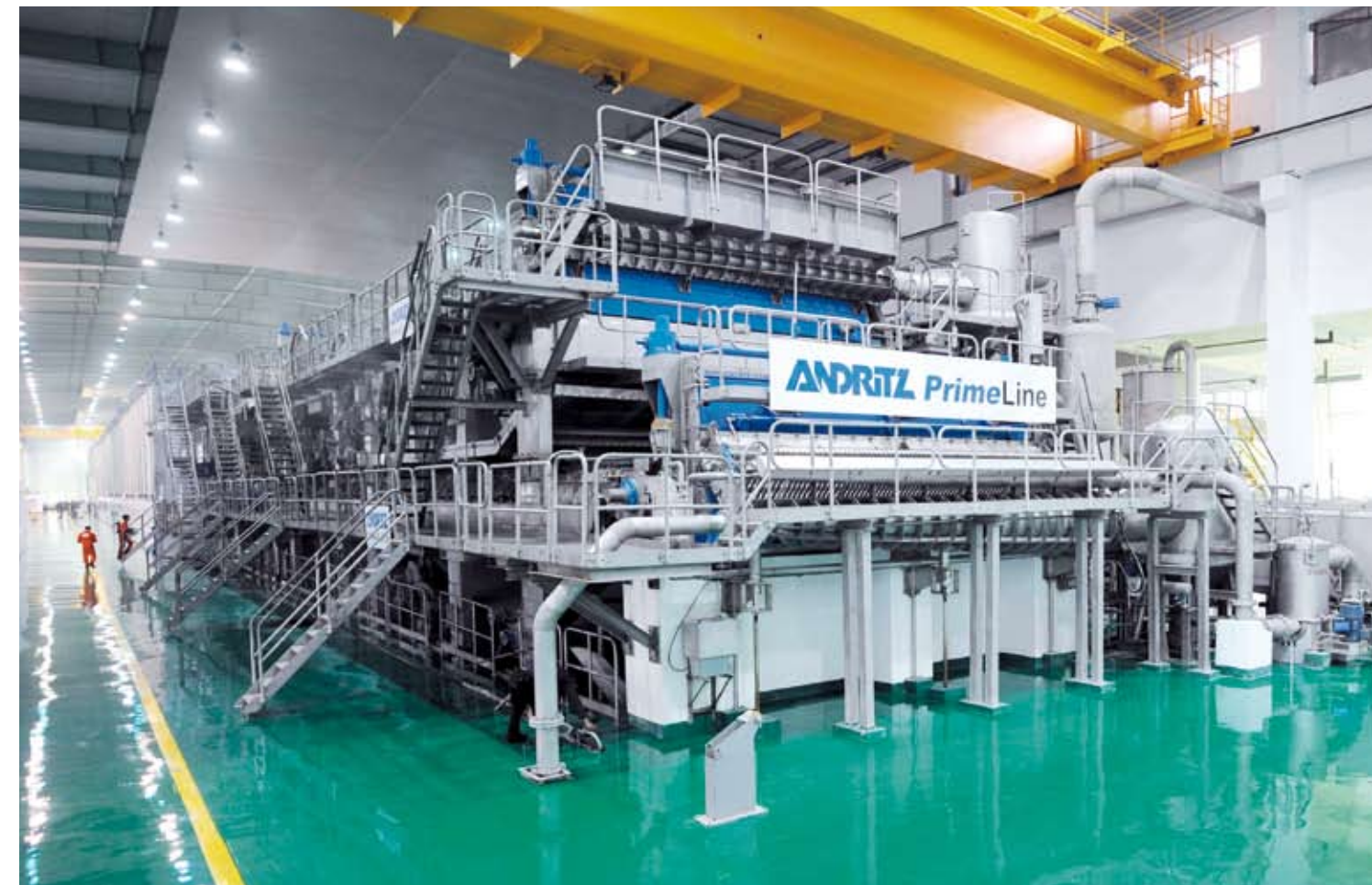
▲ PM6 is 5.6 m wide (trim width) and designed for 1,100 m/min. PM6 will bring Hebei's total capacity to 700,000 t/a, making it the largest containerboard producer in northern China.
