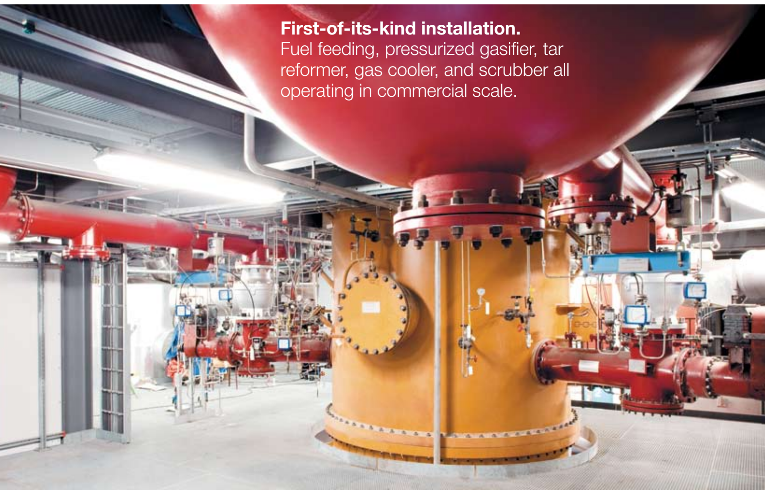
▼ The ANDRITZ Carbona gasifier is a pressurized bubbling fluidized bed (BFB) design.
