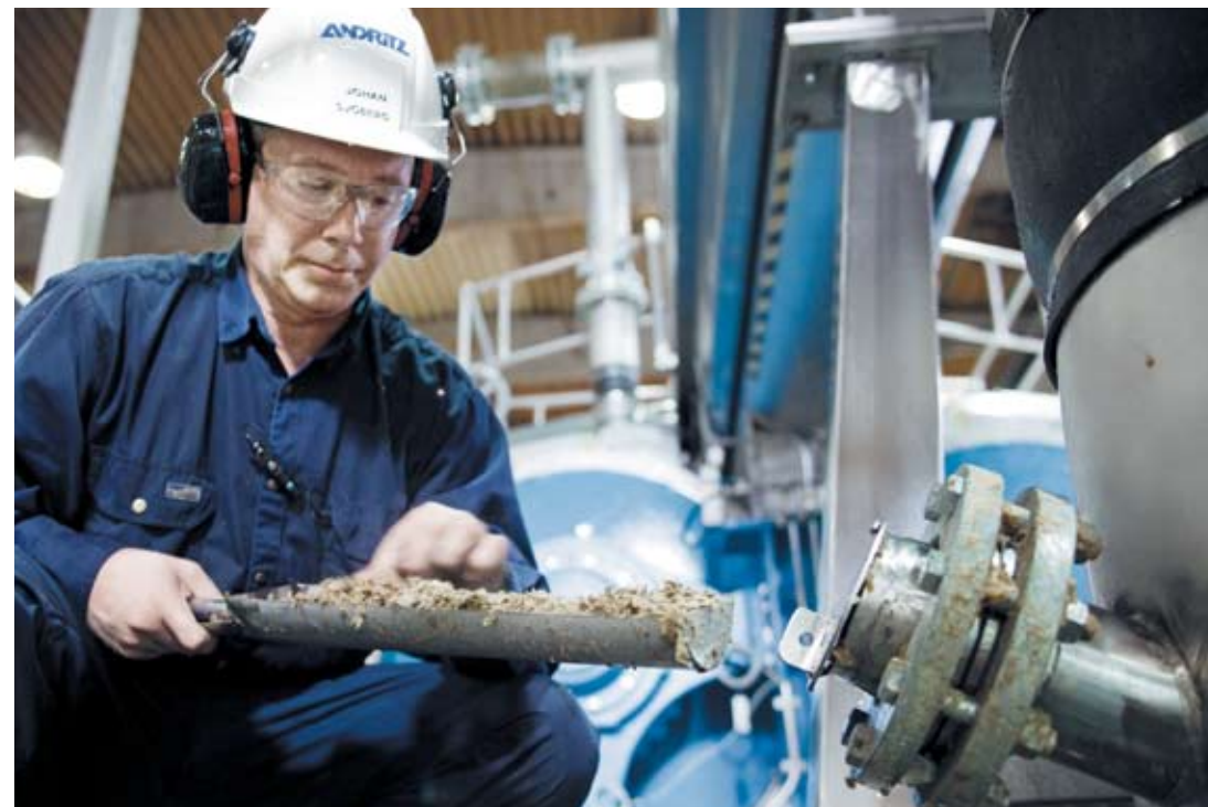
▲ Johan Sjöberg, Process Specialist with ANDRITZ, takes a sample of pulp after it is processed by the AWP and before it enters the oxygen stage.
