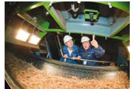
▲ Wood loss measurements provided by BarkScan™ provide the missing link for optimized debarking control. Here, Günter Flicker (left) and Rudolf Mayböck inspect the camera system utilized by BarkScan™.
