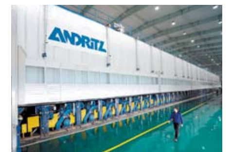
▲ The dryer section is both single-tier and double-tier and is equipped with a calender, a film press, and an air turn.
