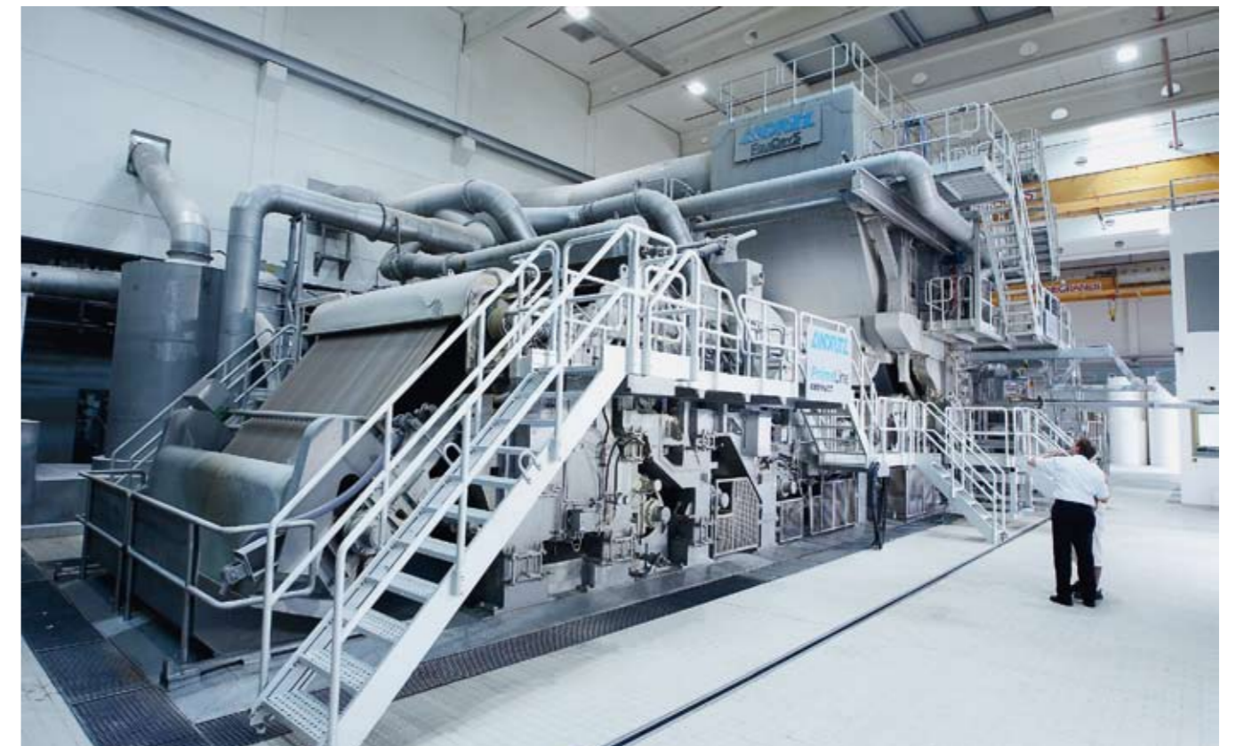
▼▲ The PrimeLineCOMPACT machine (PM6) at Fripa is configured for 30,000 t/a production with a machine speed up to 2000 m/min. The paper width is 2.75 m.
