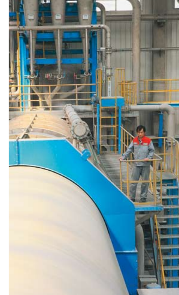
▲ The FibreFlow® drum pulper in operation at SEHT. The DIP plant started up in the middle of November 2007 and by the end of the month, the first SC paper came off the reel.
