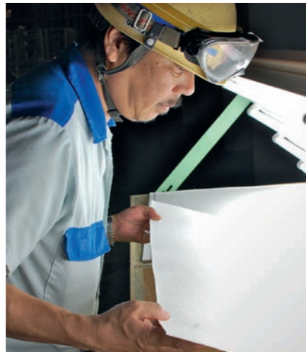
◀ Oji's Masao Fujiwara inspects a dried sheet of dissolving pulp. High-purity pulp is a must for yarn producers, whose processes are impacted by the slightest level of contaminants. Sight inspection and a series of lab test are conducted for all production.
