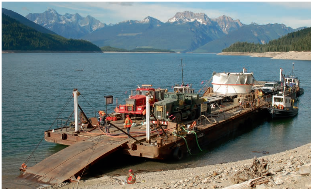
Transportation of runner for HPP Mica Dam
