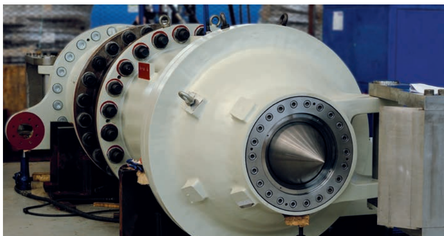
Pelton injector, HPP Coca Codo Sinclair
