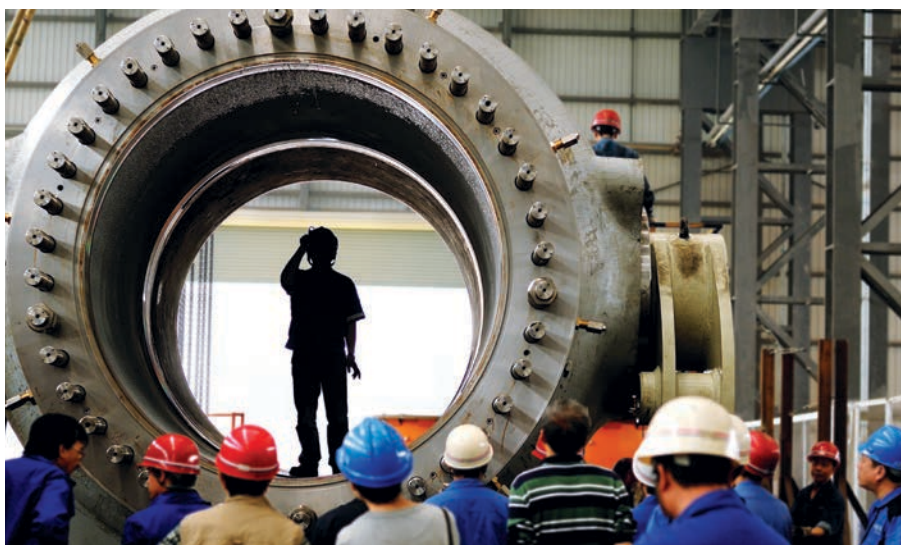
Inspection of valve for HPP Coca Codo Sinclair
